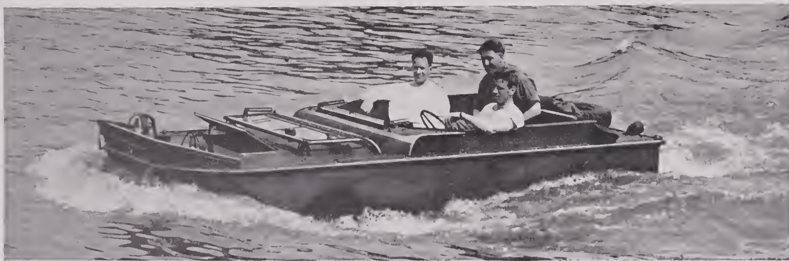
FIGURE 3. In water, final pilot model of Ford amphibious jeep achieves speed of about 6 mph.
